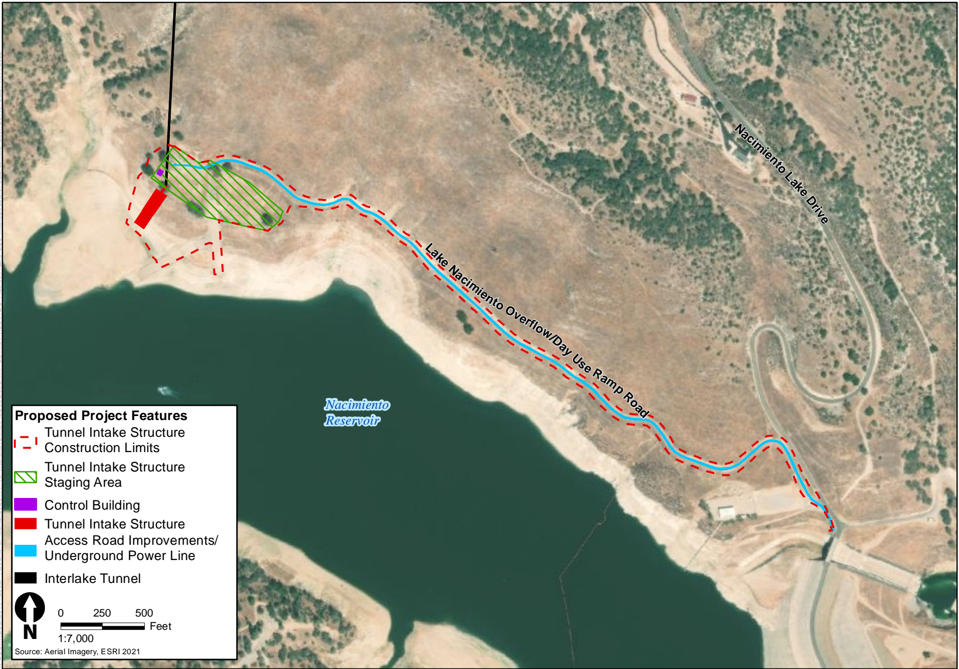
Figure ES-5 Tunnel Intake Structure and Associated Features
